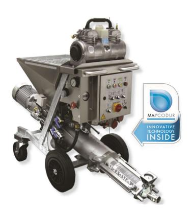
An advanced mortar mixing pump which was specifically designed for wherever heavy materials, long transport distances and/or large feed pressures are required. Delivery rate: 6 to 35 l/min with operating pressures of over 40 bar and capable of delivering to hose lengths of up to 60 metres.
