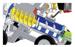
Excellent mixing quality due to the patented conveyor mixing zone and completely innovative water injection
